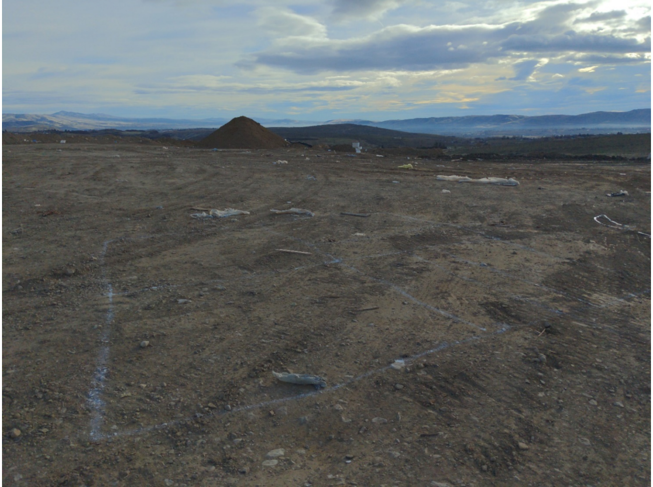
Figure A-2. Location of WAS1.1 after sampling. Each quadrant is 7.5' x 7.5'. A one-foot-wide swath was swept across each quadrant. Facing Southeast.
