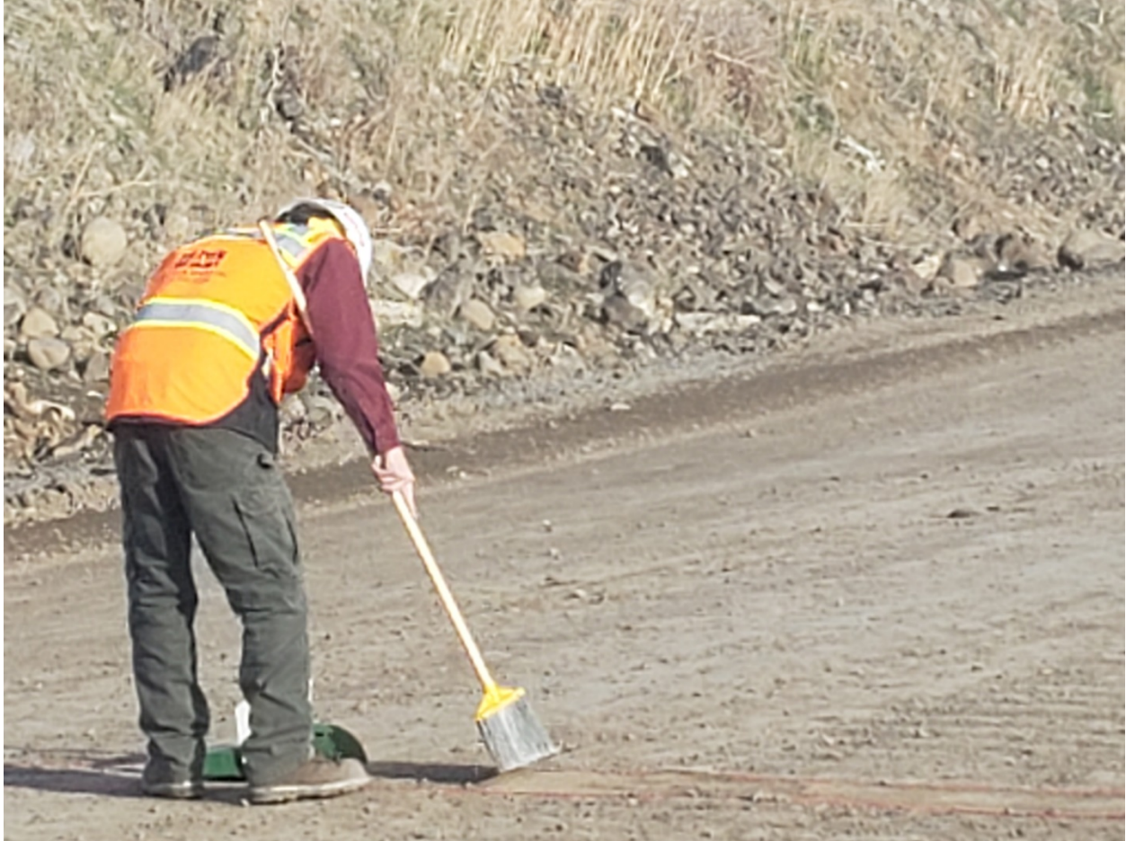
Figure A-14. Photo showing collection of a road sample courtesy of Wade Porter.
