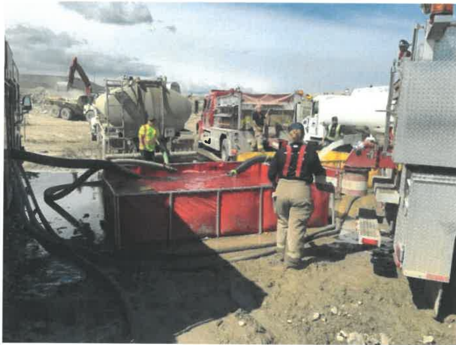
Photo 17. Tanker Water Shuttle into Husky Folding Tank at Whitehorse Fire
