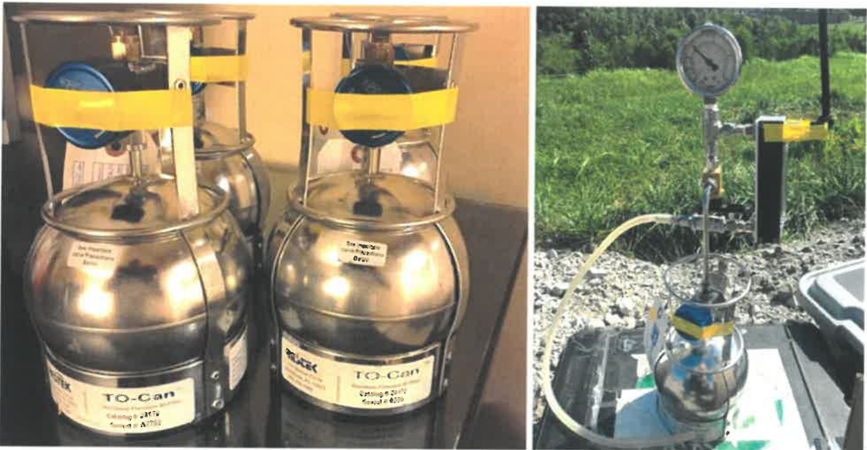
Photos A1&A2 – Evacuated TO-Cans used by LFCI for gas sampling in a previous Project
