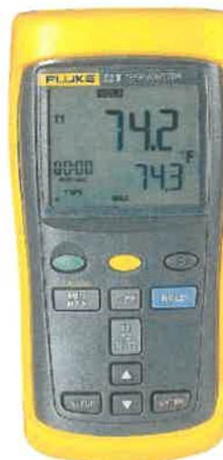
Photo 11. FLUKE 52 II used for monitoring downhole temperatures
